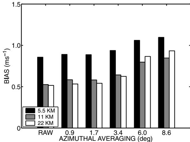
Fig. 7. Vector wind bias shown as a function of azimuthal averaging ( $\bar{\phi}$ ) used in the SO processing. The thinned raw data are marked with 'RAW'. Black (grey, white) bars indicate 5.5 km (11 km, 22 km) NWP model resolution, respectively.
