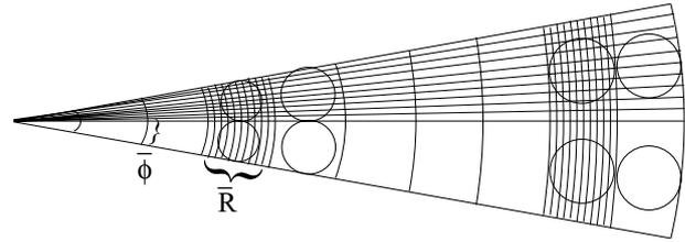
Fig. 1. Schematic illustration of SO processing.  $\bar{R}$  is the range bin spacing and  $\bar{\phi}$  is the azimuthal averaging.
