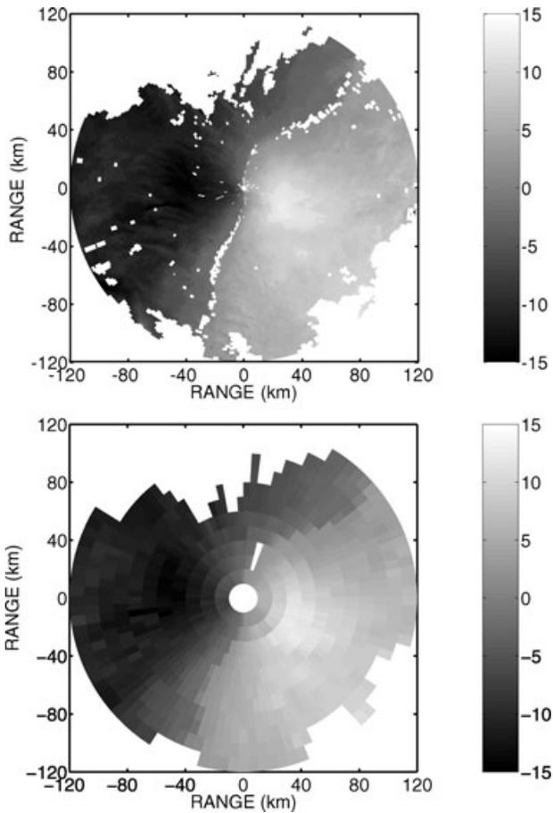
Fig. 3. Raw radar radial wind data (upper panel) and corresponding SOs generated with range bin spacing of 10 km, and azimuthal averaging of  $3.4^\circ$  (lower panel) at Karlskrona, 31 January 2002, 12 UTC.
