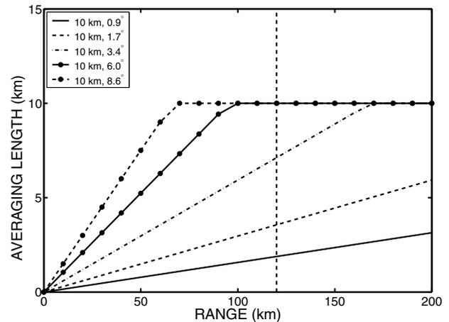
Fig. 2. Illustration of averaging lengths used in SO processing at different measurement ranges. Vertical dashed line indicates the maximum unambiguous measurement range of 120 km.
